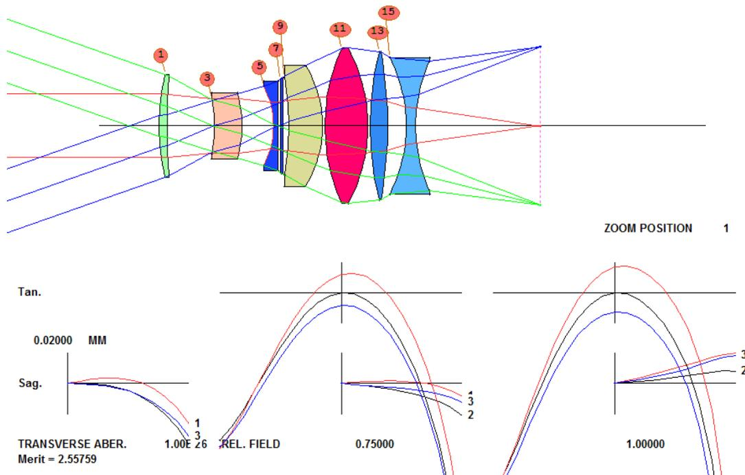
When the program splits (or adds) an element, it assigns an index pickup, because at that moment it has no other index data. In WS, change the index pickup on surface 7 to a glass model by typing
