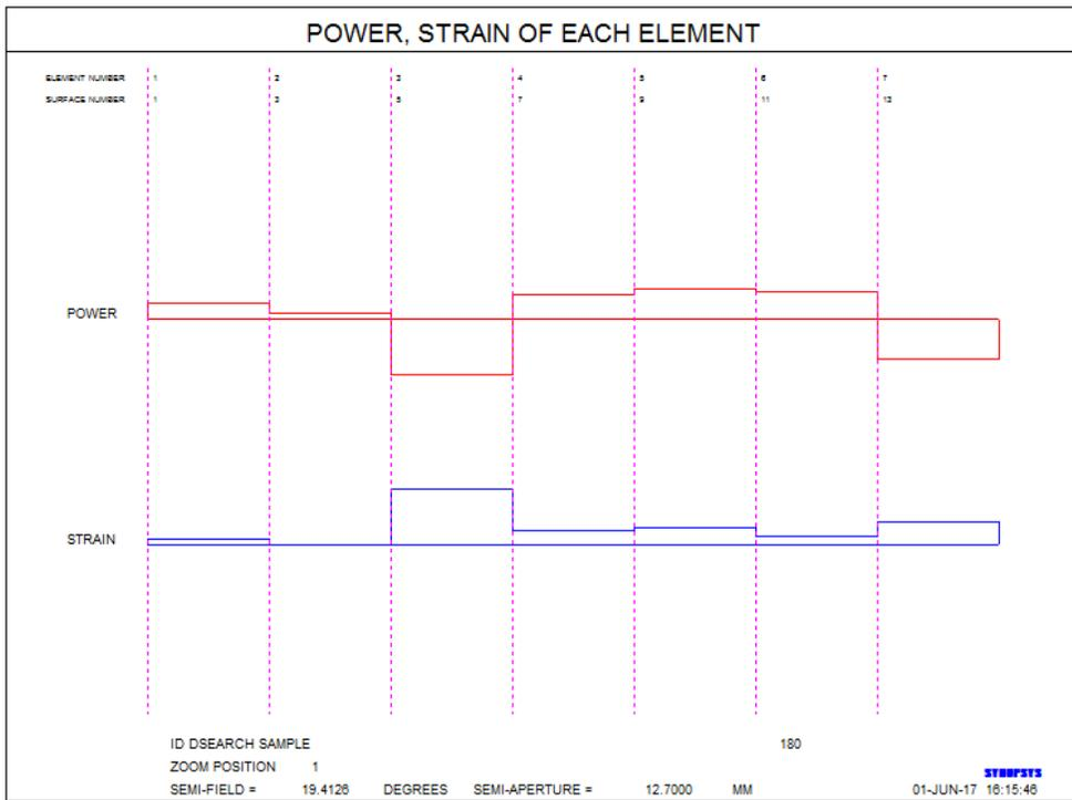
Indeed, element three has the largest strain. Now we can do one of two things: We can split that element and reoptimize, or we can use a different tool that can figure out the best place to add an element. We will try it both ways. First, let's save this version, so we can go back if things don't work out. Type
