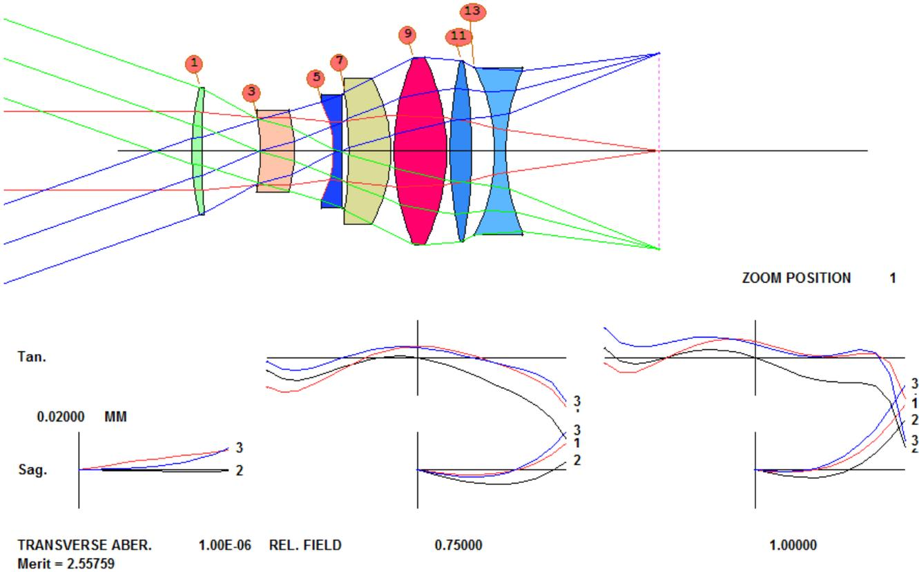
Some subtleties deserve mention: the **GLM ALL** variable will vary all glass models currently in the lens, which means all elements, since DSEARCH uses the glass model unless told otherwise. We have to control the focal length since the object height will be continuously adjusted so the image CAO is filled at full field.
