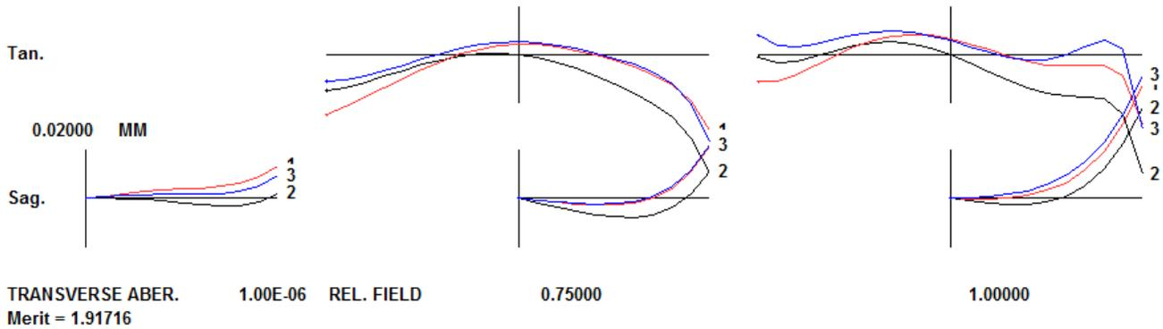
Wow! The program has inserted a new element at surface 3! And the merit function came down from about 2.55 to 1.92. There's a lesson here: The program can figure out how to improve a lens better than you can (unless you are very gifted). So it's better to let AEI do it than to try things that seem to make sense. Those things sometimes work, but AEI is better.
