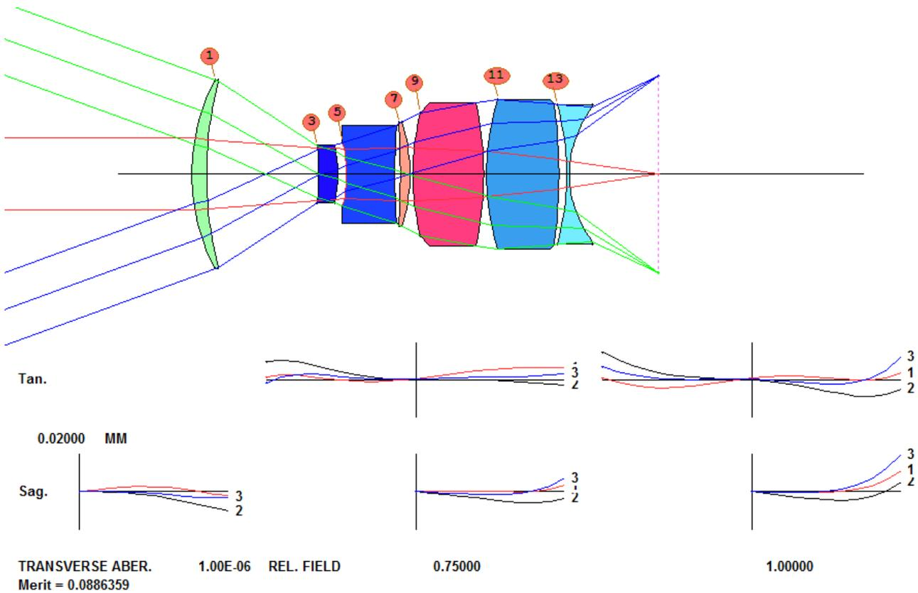
Suppose we want the lens to work over a range of object distances from one meter to infinity. There are two ways to implement that requirement: with multiconfigurations, which is very flexible but complicated, or by declaring this a zoom lens in which the object distance zooms. The second approach is better here, since it is simpler, does what we want, and we can examine intermediate object distances very easily. We have to set up this lens as a ZFILE zoom lens.
