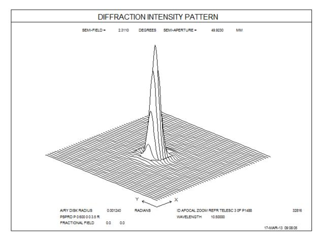
Note the value of the Airy disk radius: 0.00124. That's an angular value, since the lens is declared AFOCAL. We know that if the narcissus beam returns with an angle equal or less than that value the beam will be in sharp focus and cause a very objectionable narcissus.
