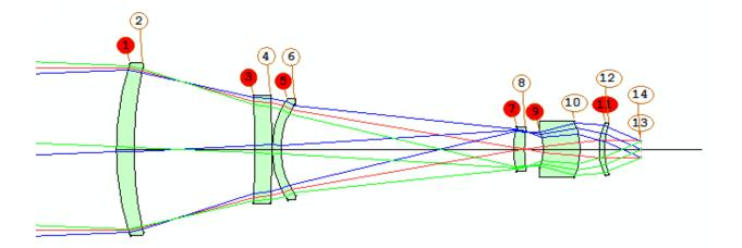
This is an infrared system, designed for the 8 to 13 um band, that uses AFOCAL mode, which means that ray output is given in *angles* instead of transverse coordinates, and the last two surfaces are flat, coincident dummies. That's where the program converts ray heights to angles, and it also marks the location of a scanning prism or other moving components that sample the image one pixel at a time. To analyze the narcissus properties of this lens, use the command **NAR**.
