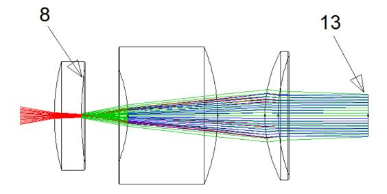
Light comes in from the left until it reaches surface 13, the flat surface on the right, which we declared a NAR surface on the dialog. (That assigns a reflection coefficient of 1.0.) We also requested a single ghost, from 13 back to 8, and from there to the last surface again. The signal flux there is collimated, and we assume that any light that returns there and is again collimated will show up on the detector sharply focused. After reflecting from 13, the rays are shown in blue, and
