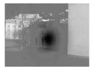
This effect occurs because at the center of the field the detector can see a ghost image of itself, reflected from a lens surface somewhere. This ghost is very cold – because the detector is very cold – and the total background signal seen by the detector is therefore lower at the center than it is at other parts of the field, where the ghost image is vignetted by other lens apertures, scanned out of the field, or so aberrated that it cannot form a sharp image.
