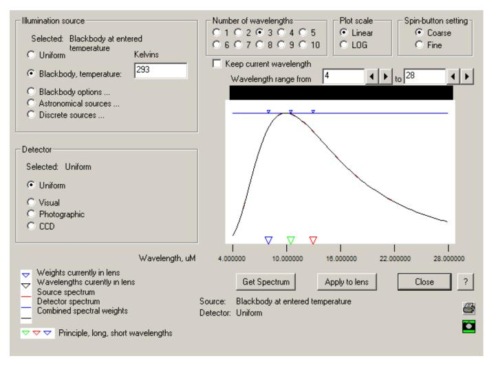
Although the atmosphere absorbs much infrared radiation, it has a window of transparency centered at a wavelength of just over 10 microns, which nicely fits the spectrum shown above.
