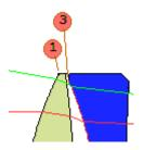
If you also want a smaller bevel on side 2, adjust it with the spin buttons for points D, and then click the **–F** button for that side to remove the flat portion.
