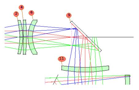
Let's assume you want it to be thicker. Either enter a larger number in the Thickness edit box or click the upper spin button on that box. The thickness increases. The amount by which the spin buttons change the dimension is given in the Spin increment box.
