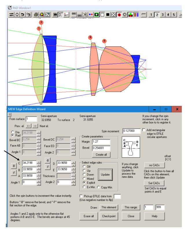
The program creates five reference points at the edge of the element, labeled A through E in the diagram on the dialog. You usually have to edit those default dimensions, and the data for element 1 show one reason why. The first surface is convex, and you may not want a bevel on that surface. The program defined the default edges and put into effect the Explicit rules, which work for most lenses and for which you can edit the data with the edit boxes and spin buttons on the dialog.
