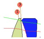
This increases the element diameter, but again has left dimensions A and B where they were. Let us reduce the size of the bevel on surface 3. To the right of the edit box for dimension B there are two spin buttons. Click the upper of the two about eleven times, watching the bevel get smaller and the flat portion getting larger. By clicking on the two spin buttons while watching the picture, you can quickly define exactly the edge you want.
