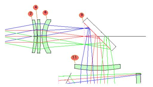
Change the increment to 0.02, click Update, and use the lower spin button in box D to add a bevel to the back side of the mirror.
