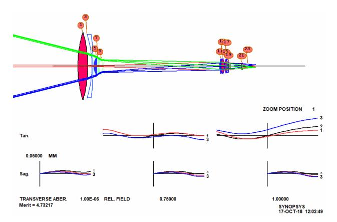
When a design has improved but won't go any further, it is a good idea to figure out why. We are suspicious of the first element, the thickest in the lens, whose edge is very thin. What is the thickness now?
