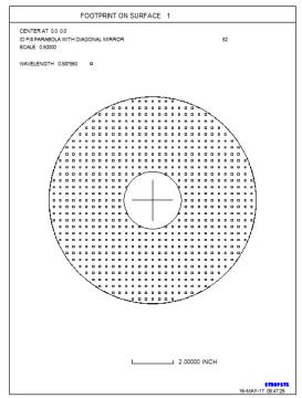
Now you see the inside aperture, which is free of rays. Here's a neat trick: suppose you don't know where the rays are being vignetted (that happens sometimes with complex lenses). Here's how to find out: First hit the <Enter> key (when you have used a dialog to run anything, you go right back there. That's a time-saver). Now, click the Switches button
