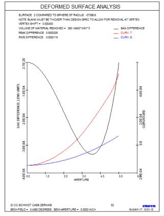
The black curve in the above picture shows how the surface departs from the closest-fitting sphere, which in this case is very close to flat.
