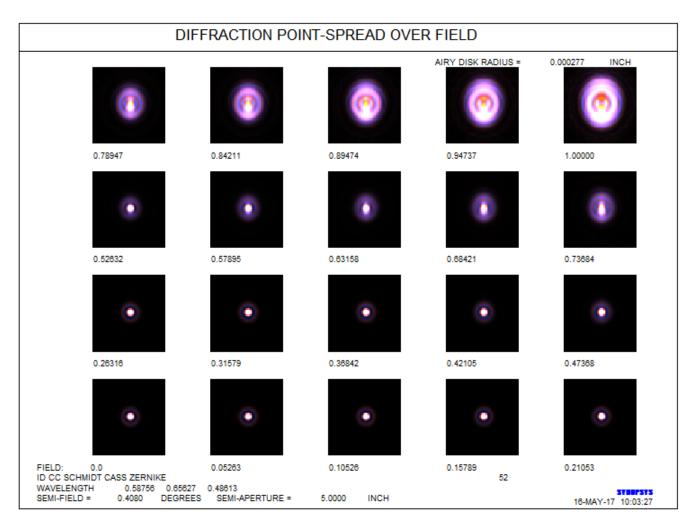
The image at the lower left is the on-axis image, while the upper right is the edge of the field. That's not too sharp. Let's examine it in a different format. Back in MPF, select the option to **Show as surface**, and change the Height from the default 1 to 0.
