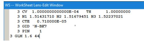
We are going to vary the glass types in order to correct color, and we don't want surface 3 to always pick up the index values from surface 1. So we assign it a glass model of its own, somewhere in the flint part of the glass map. Now type, in the edit pane.
