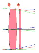
The program has removed the YMT solve from surface 2 and added an index pickup on surface 3 (3 **PIN** 1). Click on surface 3, and type 3 **GLM** 1.6 44 in the edit pane. Then click the Update button.
