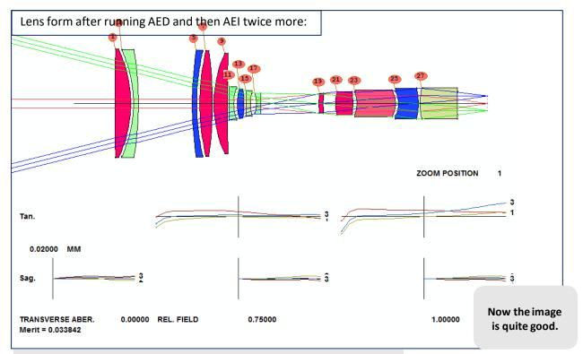
Note that the ray fan plot scale changes 0.05mm to 0.02mm in this design.
